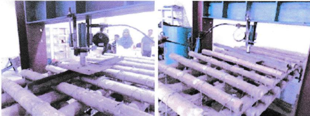
Fig. 7. Loading tests on bamboo mattress.
